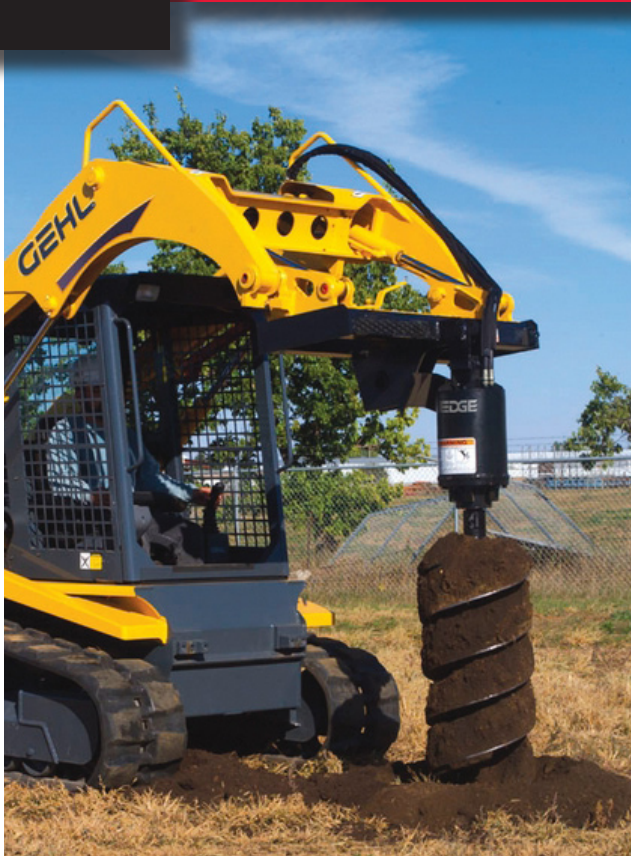
Used on a tracked skid steer, EDGE planetary augers are great in landscaping applications.
