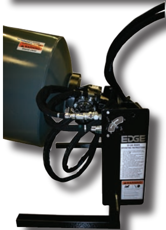
Direct hydraulic drive of gearbox.
