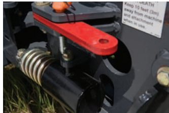
Locking pin for transport, and pivot springs allowing tight turning radius.
