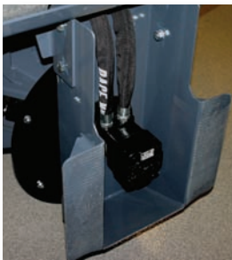
Easy access to hydraulic motor.
