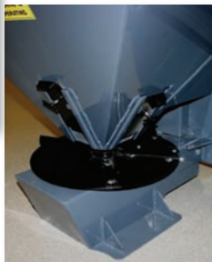
Adjustable gates control flow.
