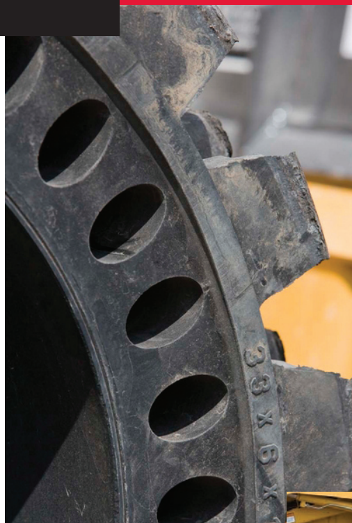
Elliptical holes provide pneumatic-type ride.
